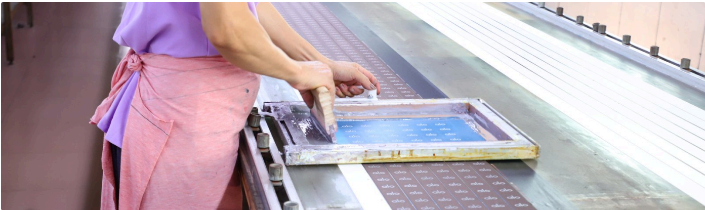
Screen printing a repeating brand label onto satin tape, printing workshop.
